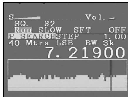
Figure 8—The AR7000B band scope in the search mode. The band limits, search name (40 Mtrs in this example), mode, step size, bandwidth, sweep direction and pause duration can all be varied in a setup menu.
